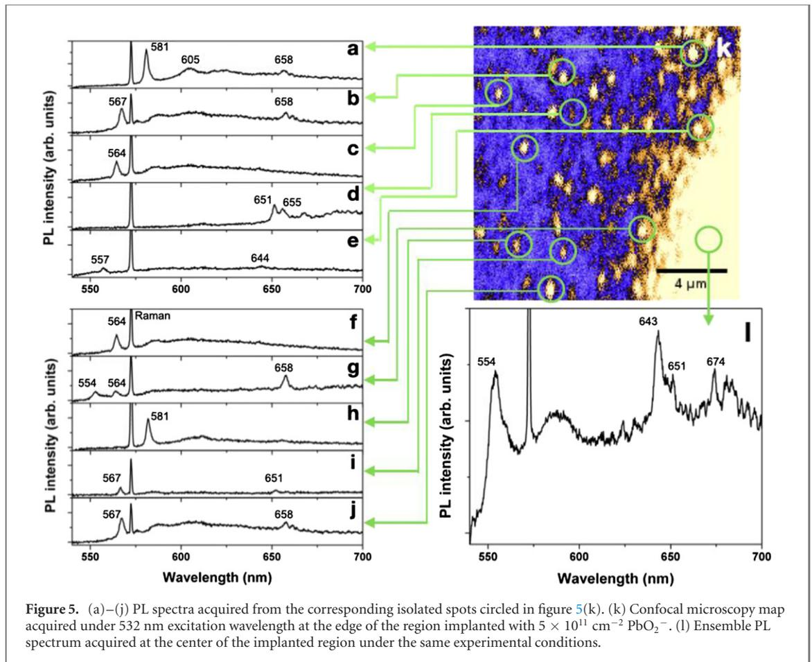
**Figure 5.** (a)–(j) PL spectra acquired from the corresponding isolated spots circled in figure 5(k). (k) Confocal microscopy map acquired under 532 nm excitation wavelength at the edge of the region implanted with  $5 \times 10^{11} \text{ cm}^{-2} \text{ PbO}_2^-$ . (l) Ensemble PL spectrum acquired at the center of the implanted region under the same experimental conditions.
