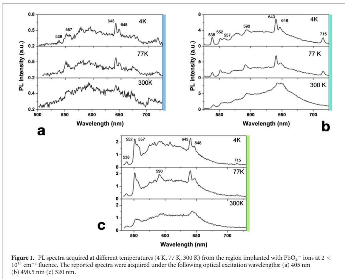
**Figure 1.** PL spectra acquired at different temperatures (4 K, 77 K, 300 K) from the region implanted with  $\text{PbO}_2^-$  ions at  $2 \times 10^{13} \text{ cm}^{-2}$  fluence. The reported spectra were acquired under the following optical excitation wavelengths: (a) 405 nm (b) 490.5 nm (c) 520 nm.
