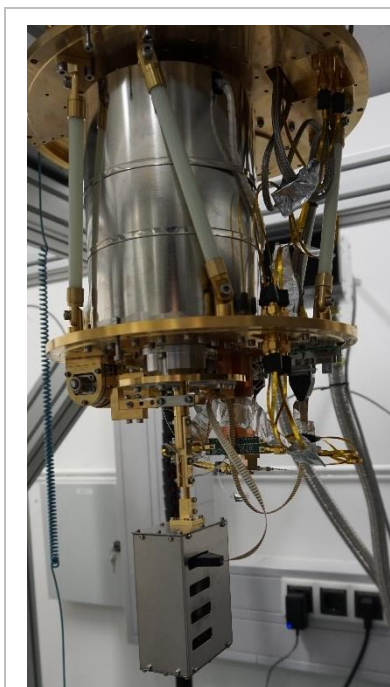
Figure 57: View into the cryostat: The large silver 'bin' in the upper part is the Niobium shield around the superconducting ADR magnet; the TES are mounted inside the Titanium box in the lowermost part, which is connected to the FAA cold finger.
