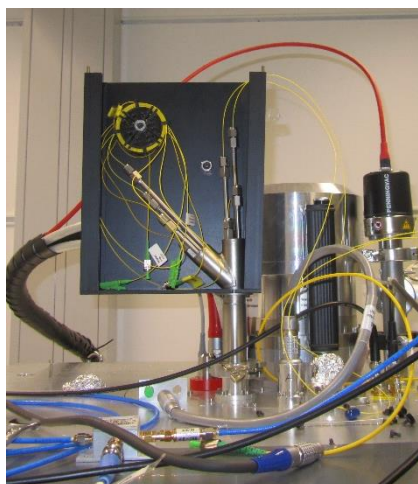
Figure 58: Home-built fibre vacuum feedthrough into the cryostat, accommodating up to eight fibres.
